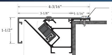
Note: Drill an oversized hole in the cover allowing for the screw to fit up to the frame. This will allow for the cover to be removed by removing only the cover screw.
