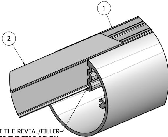
INSERT THE REVEAL/FILLER INTO THE ZERO REVEAL POSITION. SLIDED IT UP INTO THE POST.
