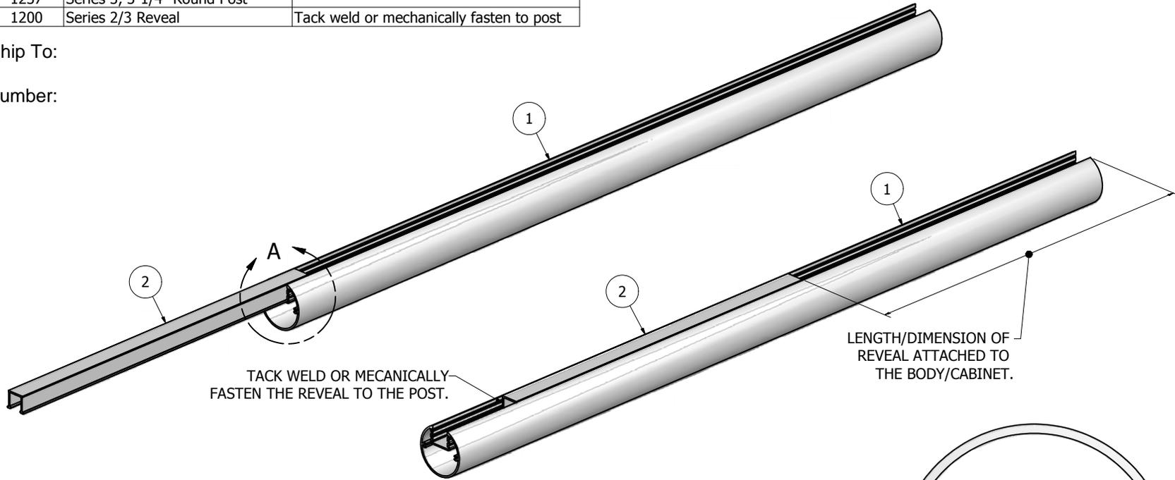
TACK WELD OR MECHANICALLY FASTEN THE REVEAL TO THE POST.
