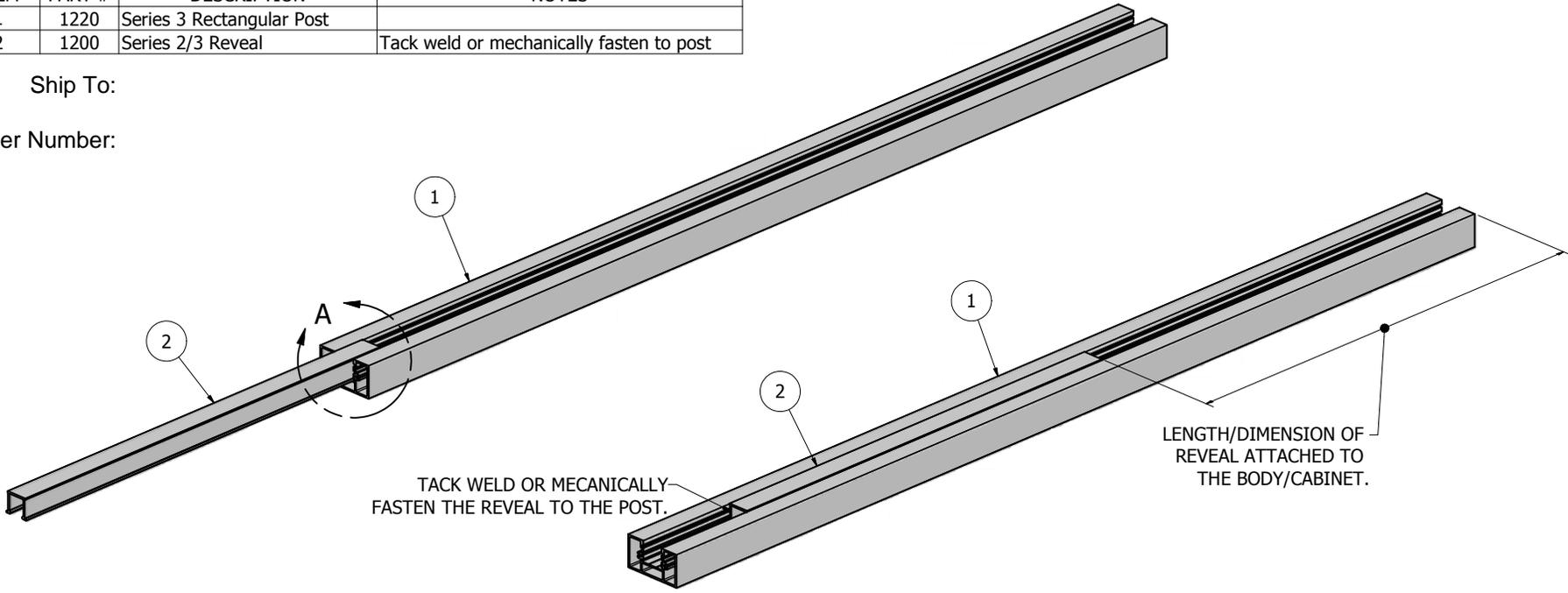
TACK WELD OR MECANICALLY FASTEN THE REVEAL TO THE POST.
