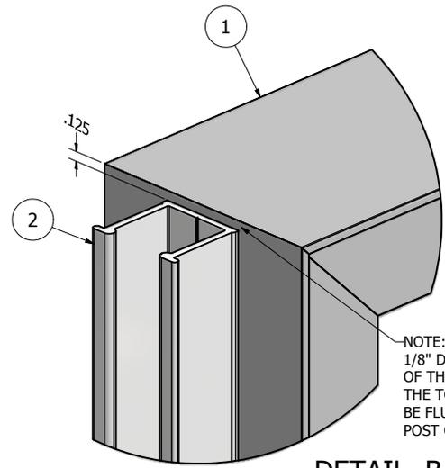
NOTE: THE REVEAL IS PLACED 1/8" DOWN FROM THE TOP OF THE CABINET THE ALLOWS THE TOP OF THE CABINET TO BE FLUSH WITH THE TOP OF THE POST CAP.
