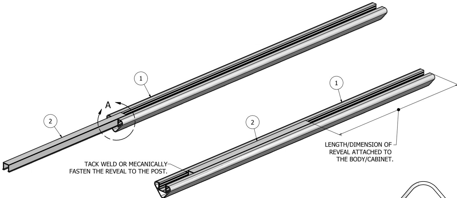
TACK WELD OR MECHANICALLY FASTEN THE REVEAL TO THE POST.
