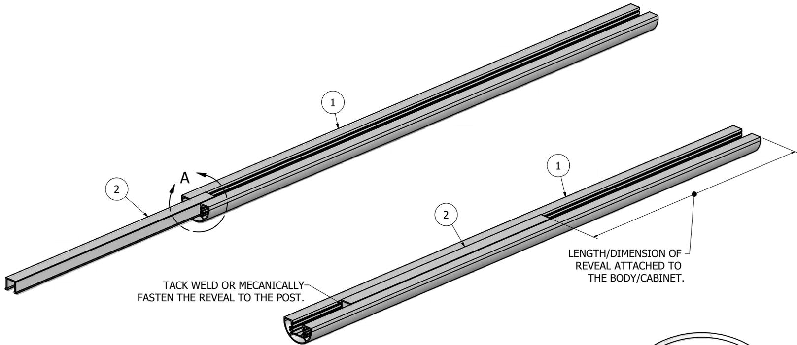
TACK WELD OR MECANICALLY FASTEN THE REVEAL TO THE POST.
