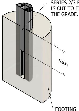
SERIES 2/3 REVEAL/FILLER IS CUT TO FIT 6" BELOW THE GRADE.
