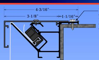
Note: Drill an oversized hole in the cover allowing for the screw to fit up to the frame. This will allow for the cover to be removed by removing only the cover screw.
