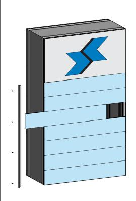
Insert Panels slide in and out after Insert End Cover is removed
